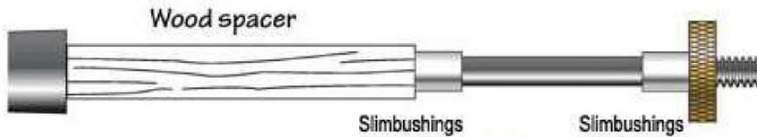
Advance a 60° revolving cone center into the dimpled end of the mandrel and tighten using light pressure. Do Not over tighten the tailstock or mandrel nut as this may cause the mandrel to flex resulting in off-center barrels.
